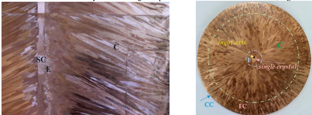
Figure 5. Structural zones as revealed on: a/ longitudinal section; b/ cross-section of the brass ingot.
