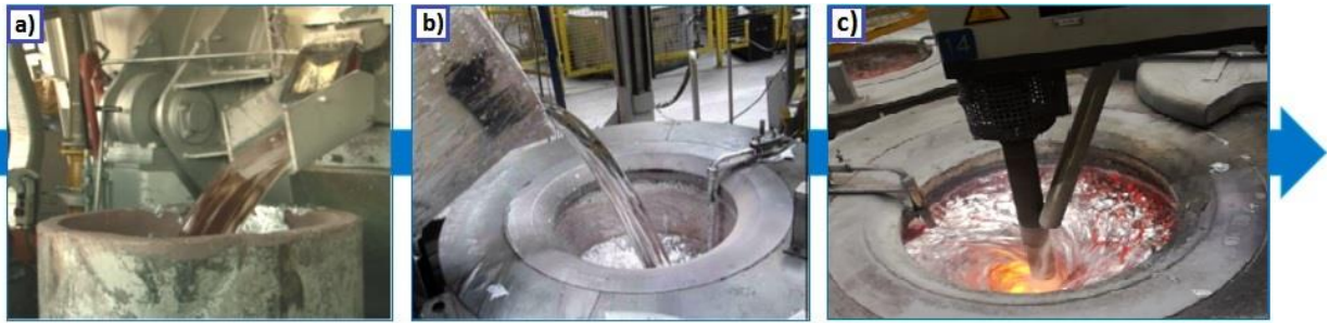
Figure 1. The stages of melt preparation: a) pouring from melting furnace, b) melt transport to holding furnace, and c) melt processing
